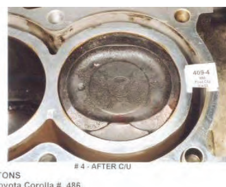
Picture I - Piston after P.i. treatment
