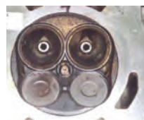
Combustion chamber before P.i. treatment.
